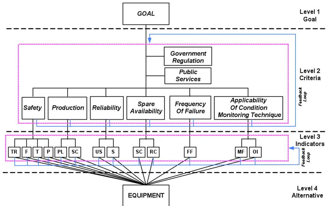
Figure 2. Hierarchy Structure of Combination Model of Serial and Parallel
