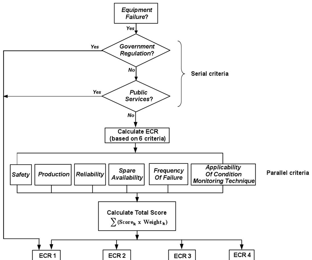
Figure 1. Combination Model of Serial and Parallel
