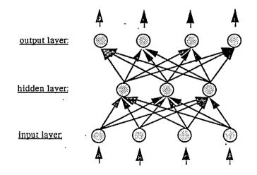
Figure 2. Feedforward layered network
