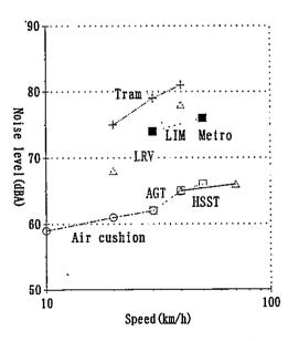
Although it is advanced to be low noise for LRVs, it is not so low noise in the same speed regions in contrast to other new urban transportation systems. As to electromagnetic field in the vehicle it is not so high level for LRVs, but has different features in damping characteristics with distances that the level on around ceiling is higher than the floor in the vehicle because of installing electric devices on the ceiling.
