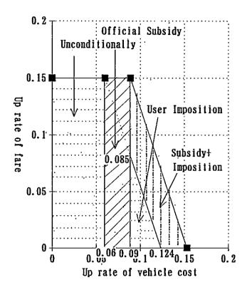
Fig. 6 Permitted cost up ratio of vehicle in introducing LRVs
