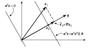
Figure 3.1. Projecting a vector on a normal to a plane
